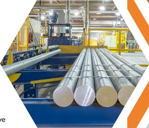
Aluminium Shapes is one of only two UK-owned aluminium extrusion companies, operating from a 70,000 sq. ft. facility in Corby, Northamptonshire. In addition to two six inch extrusion presses, Aluminium Shapes boasts extensive on-site fabrication facilities including standard cutting, double headed mitre cutting, CNC machining up to 6500mm lengths, and punching facilities.
